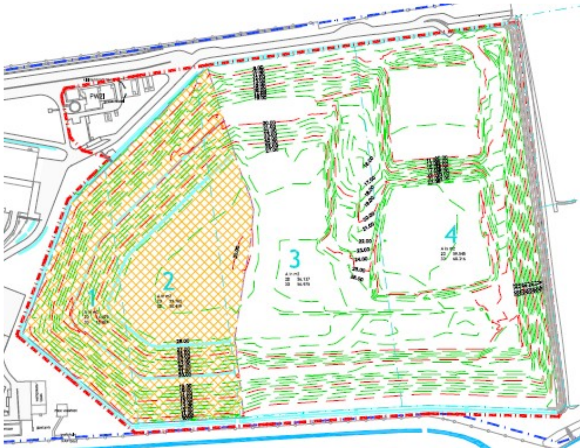
Figure 2: Top cover at De Kragge 2. The lined part of the landfill is shaded.
